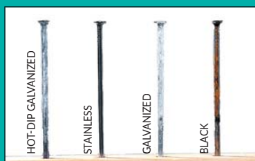
Nail samples after 96 hours (4 cycles) in the Kesternich chamber
