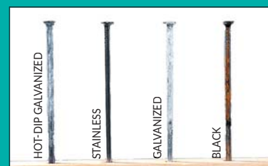
Nail samples after 168 hours (7 cycles) in the Kesternich chamber
